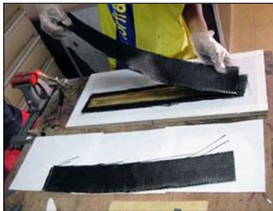
Figure 3: Typical Photographs of Composite through the Hand Layup Process.
