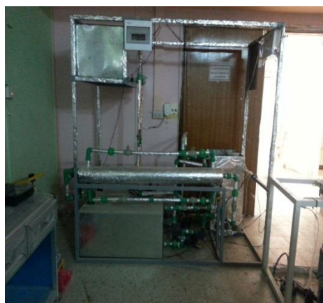
Fig. 2. The heat exchanger
