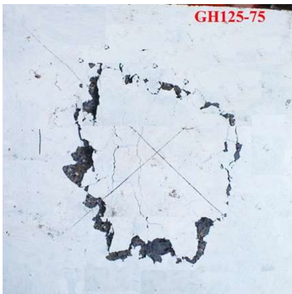
Figure 5. A Typical cracks patterns on the bottom face of tested specimens
