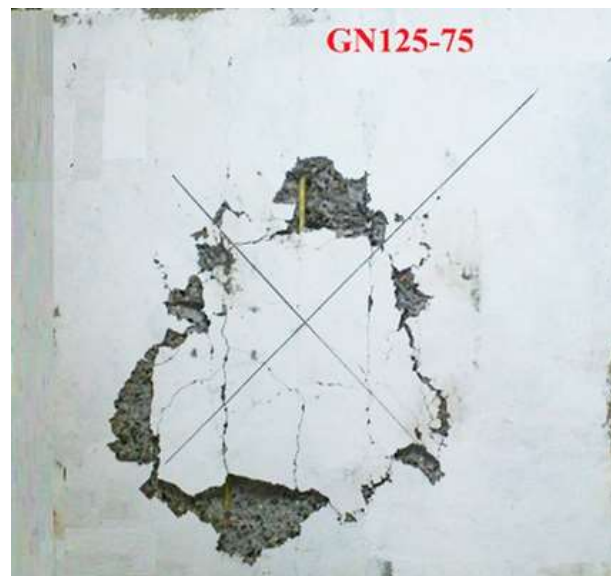
Figure 5. A Typical cracks patterns on the bottom face of tested specimens
