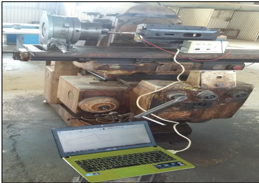
Fig 2. The connection of shaping tool with interface and monitor.
