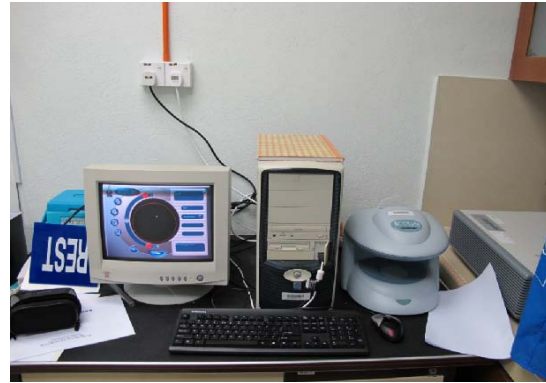
Figure 4: aCOLyte colony counter connected to the computer.
