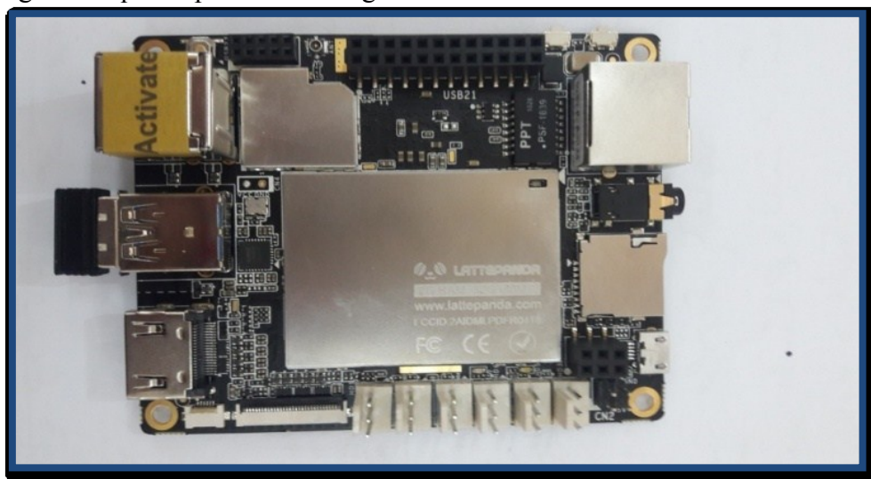
Figure (6) : LattePanda Microprocessor of Quadcopter Designed.
