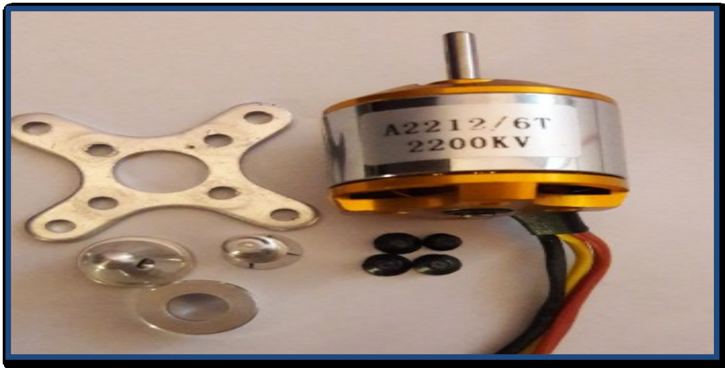
Figure (3): Brushless Motor of Quadcopter Designed
