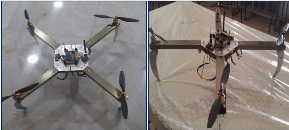
Figure (1) : Frame (x) of Quadcopter Designed
