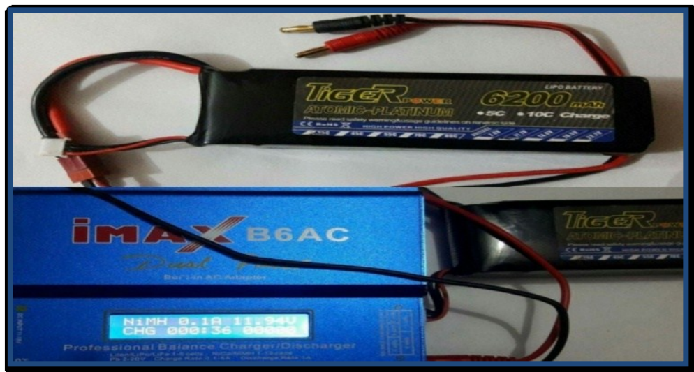
Figure (5): Lithium-Polymer (LiPo) Battery of Quadcopter Designed
