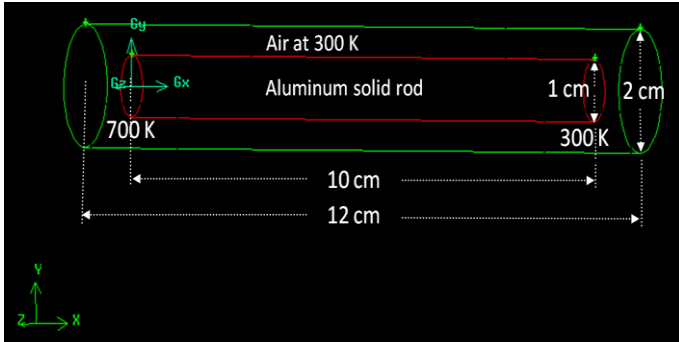
Fig.1. Sketch of the Aluminum rod and the air computational domain.
