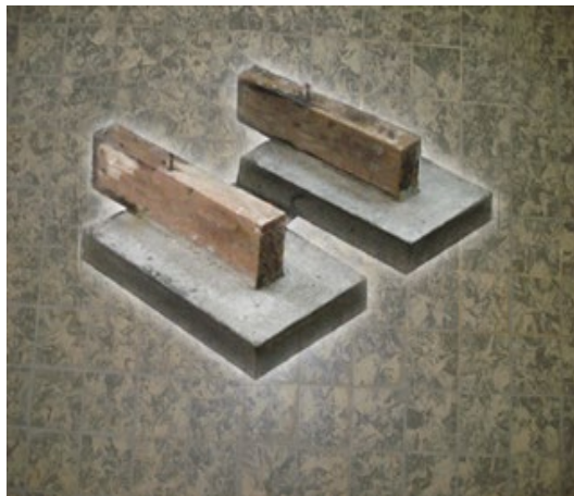
Figure 2: The casting of the first slab for push-out specimens
