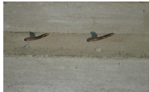
Figure 8: Bending of connectors after failure in push-out test
