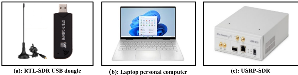
Figure 2: The essential adopted SDR hardware components for MSKU3-based CSS, (a): RTL-SDR USB dongle,(b): Laptop personal computer, (c): USRP-SDR
