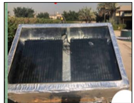
C. The solar collector is tilted at an angle of 33.2° from the horizon (latitude of the city of Baghdad)
