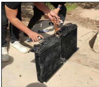
A. Heat exchangers
