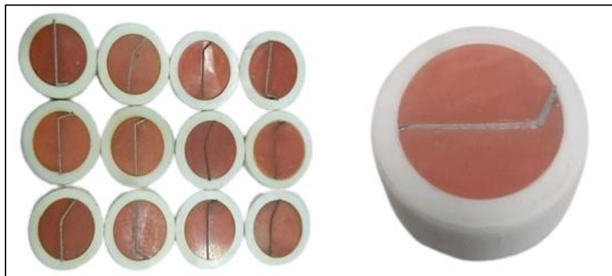
Figure 11: Micro hardness samples preparation and mounting
