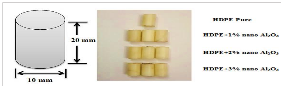
Figure 2: Standard and actual wear test specimens
