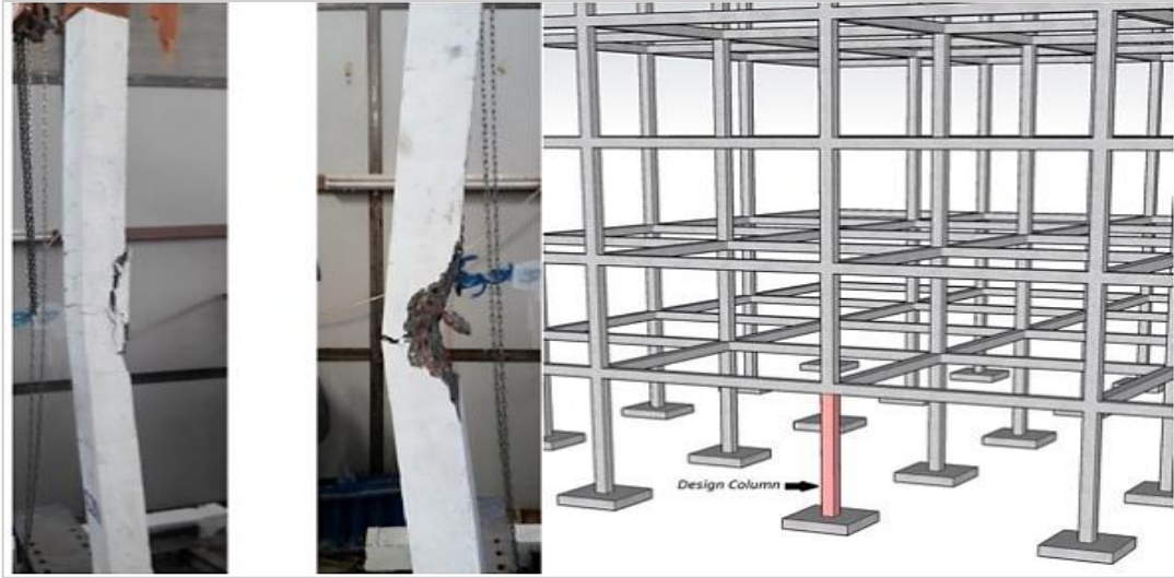
Figure 1: Collapse and failing of slender columns; Slenderness Effects for Concrete Columns in Sway Frame- Moment Magnification Method (CSA A23.3-19) [1]
