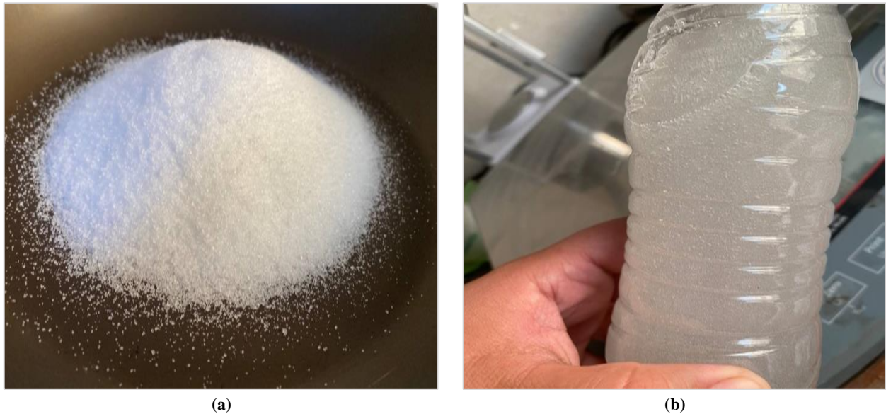
Figure 4: Polyvinyl Alcohol solution (PVA) solution preparation.
