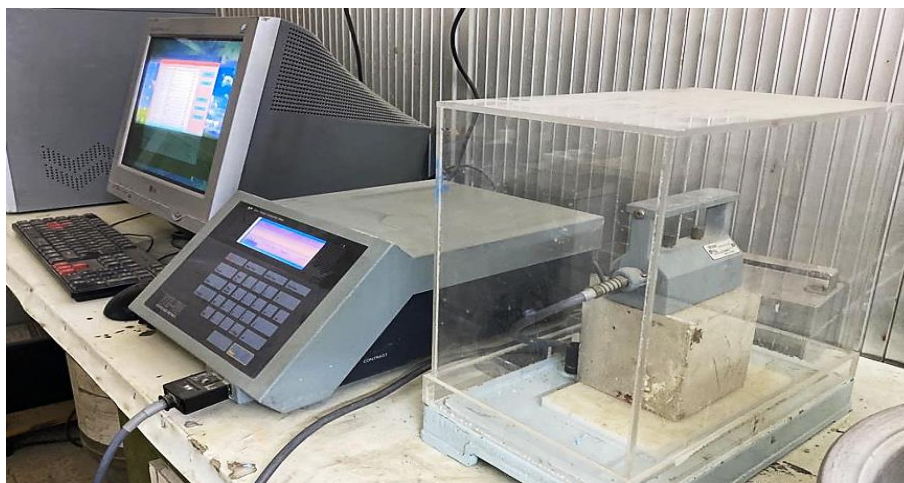
Figure 9: Thermal conductivity test by using cube (100×100×100) mm
