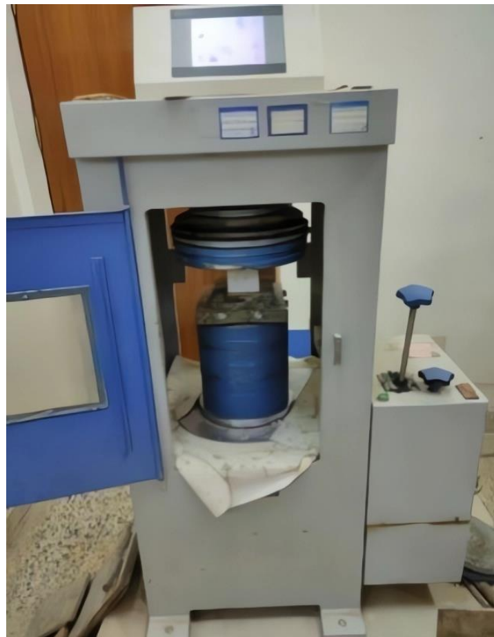
Figure 9: Compressive strength testing mechanism
