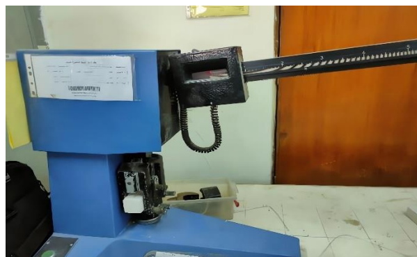
Figure 11: Modulus of rupture testing mechanism
