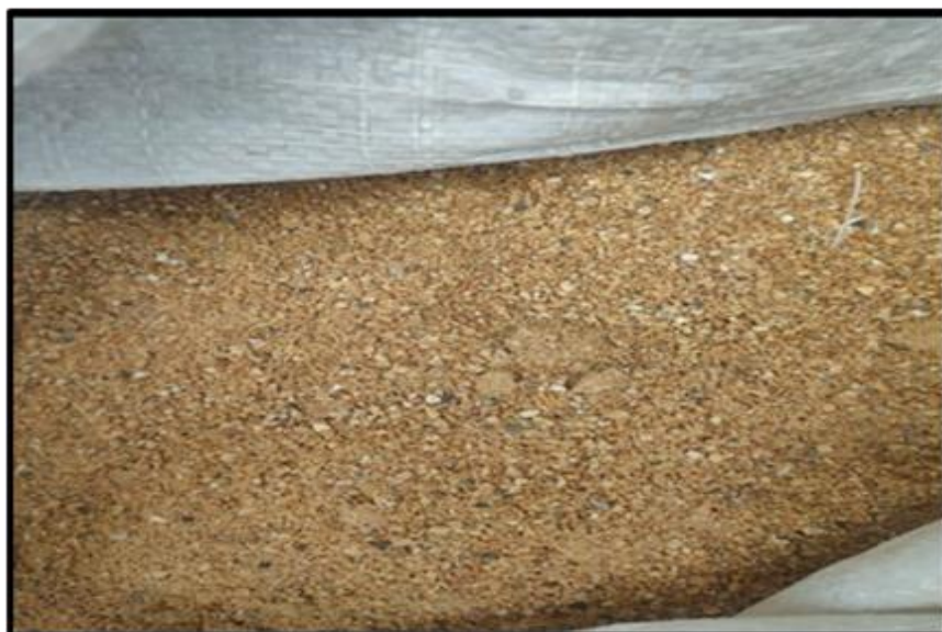
Figure 2: Crushed alumina bricks as aggregate
