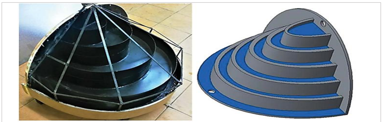
Figure 9: The spherical still after manufacturing and the Three-dimensional view [85]
