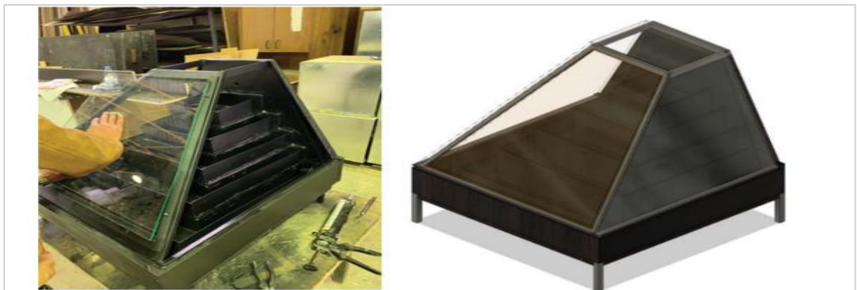
Figure 8: The pyramid still after manufacturing and the three-dimensional view [85]
