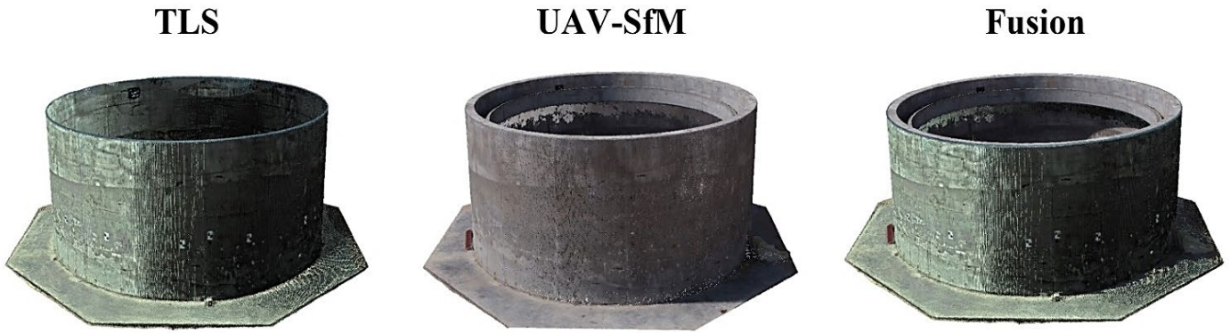
Figure 7: Fused 3D model of the tank using a co-registration approach
