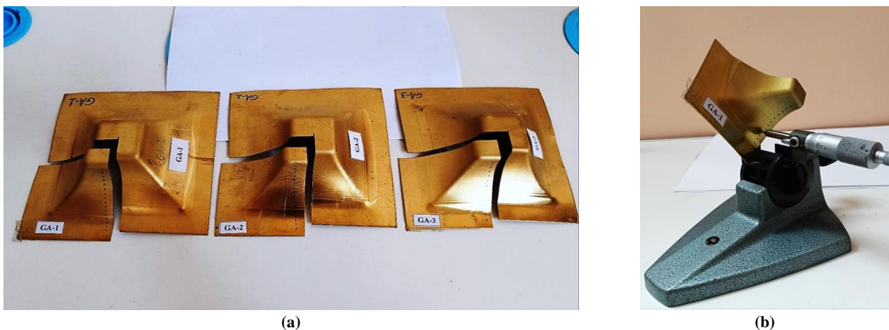
Figure 9: (a) cutting out a section from the formed part, (b) Measurement of the thickness distribution along the wall of the formed part using point micrometer
