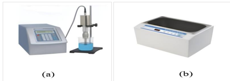
Figure 6: Ultrasonic types, (a) probe (b) bath [57]
