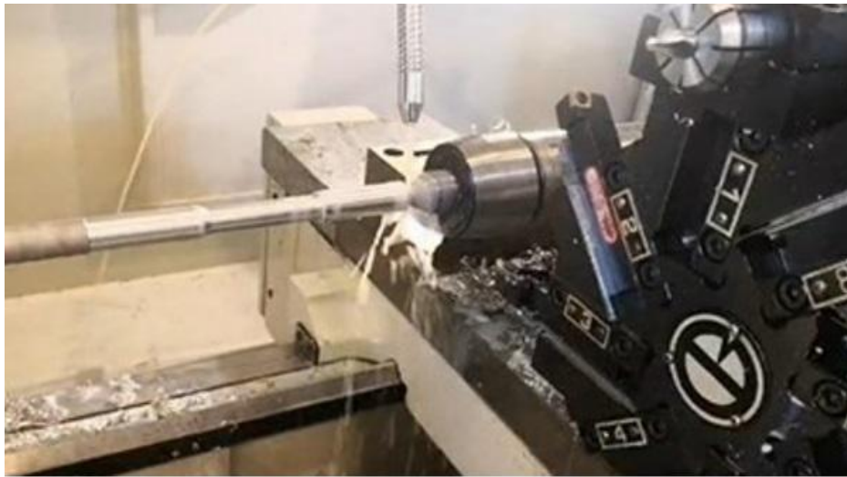
Figure 3: Tensile test specimens are manufactured in Sulaimani Technical Institute using a CNC turning machine
