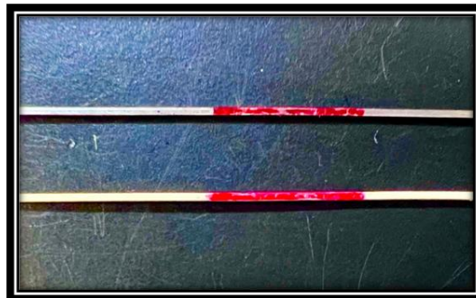
Figure (4): The portion of the wire's outer surface that did not come into contact with the bracket slot is marked with a marker to indicate the area that slid along the slot.
