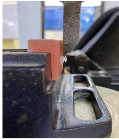
Figure (3): Debonding of the bracket
