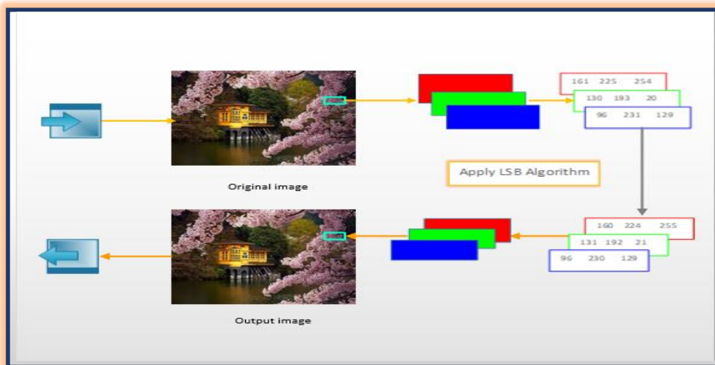
Figure(1): Block diagram to explain LSB algorithm in color image
