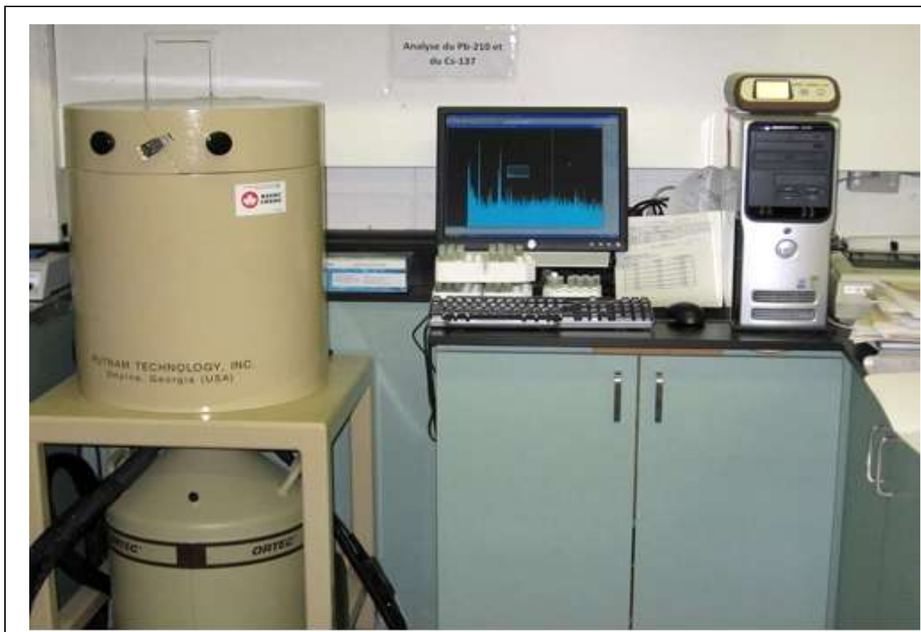
Fig(1) HPGe system for the counting of radionuclides
