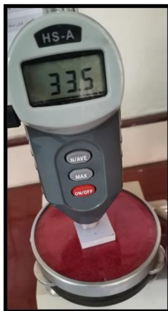
Figure 4: Shore A hardness testing.
