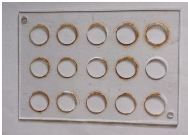
Figure 2: Acrylic mold for bacterial adherence test.
