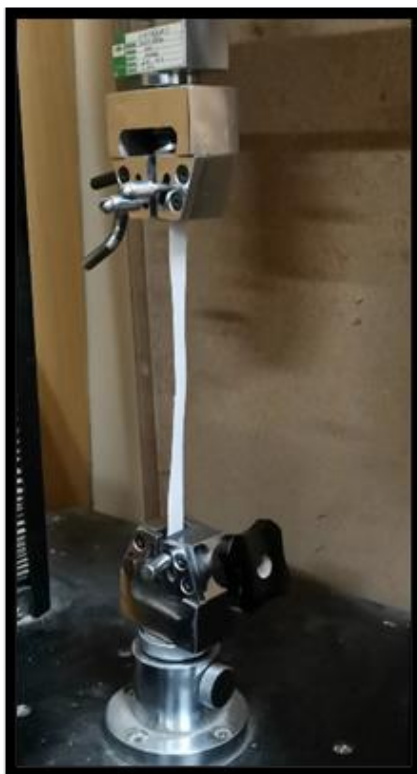
Figure 3: Tear strength test.
