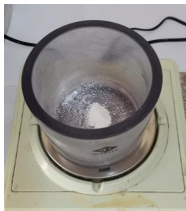
Figure 3: MCC powder added first to be mixed with silicone base.
