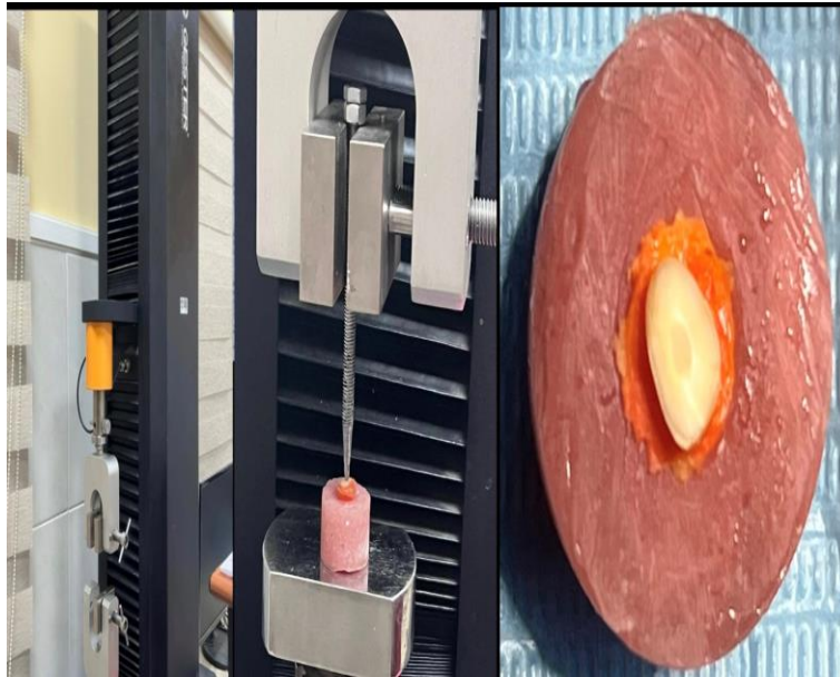
Fig. (5): A universal testing machine using a steel spherical tip with a diameter of 2 mm was aligned at the center of the canal opening of each specimen.
