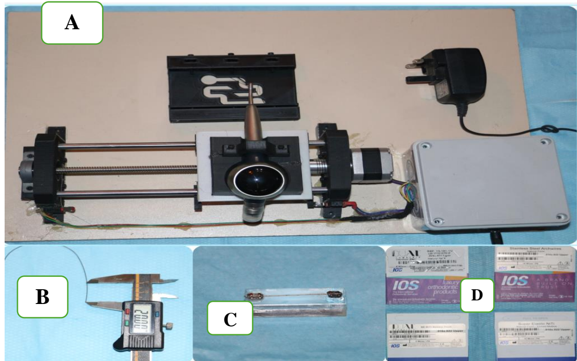
Figure 1: A: customize holding device for air polishing, B: length of wire that used, C : CNC block with wire attached to it , D : Arch wires that used.
