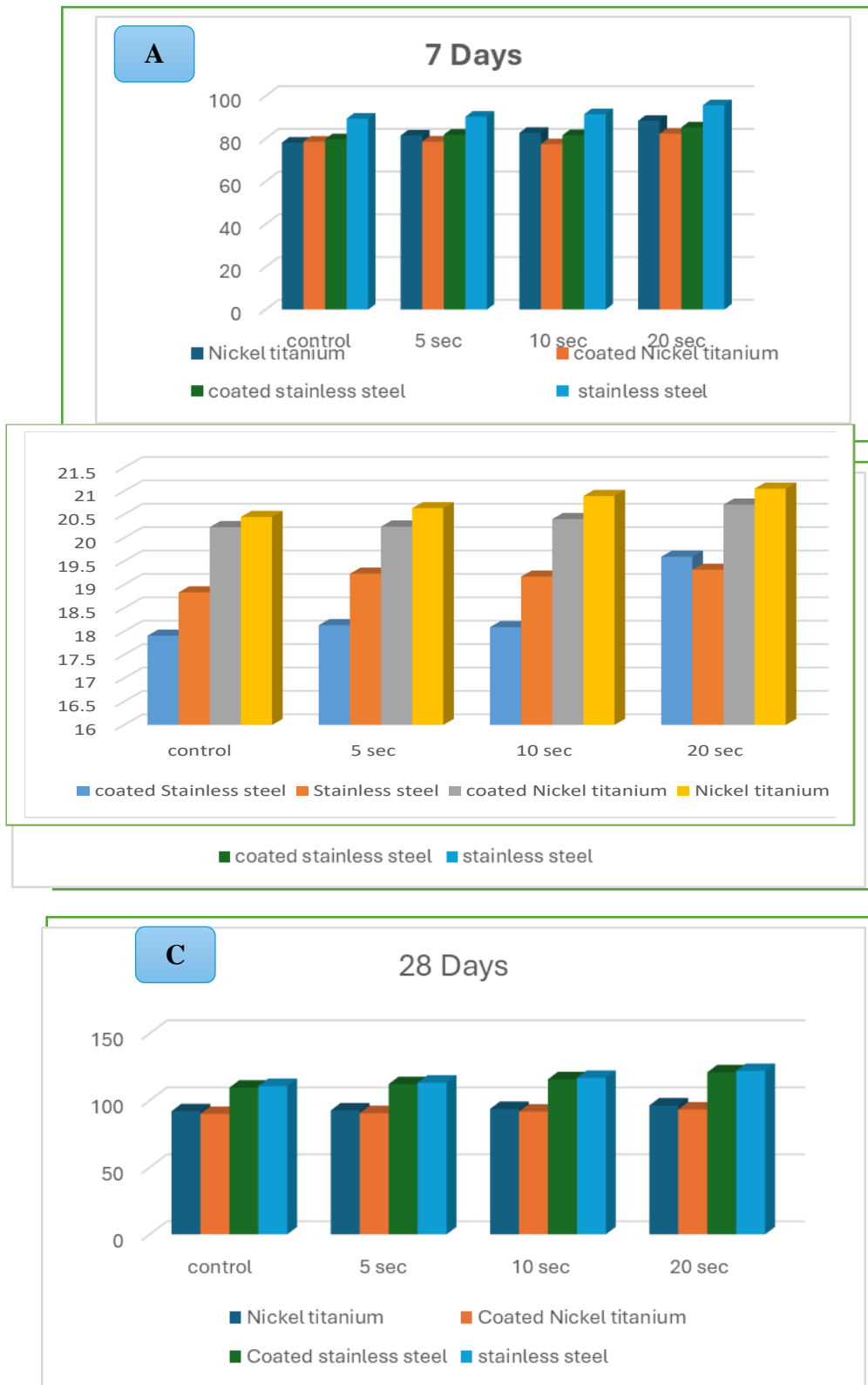
Figure 2: A -B- C: Histogram represents the effect of polishing time on the accumulative Ni ion release of different arch wire types in normal pH 6.75 media, Figure A: 7 Days , Figure B : 14 Days , Figure C : 28 Days incubation.
