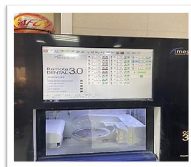
Fig. (2): The disc's wet milling procedure
