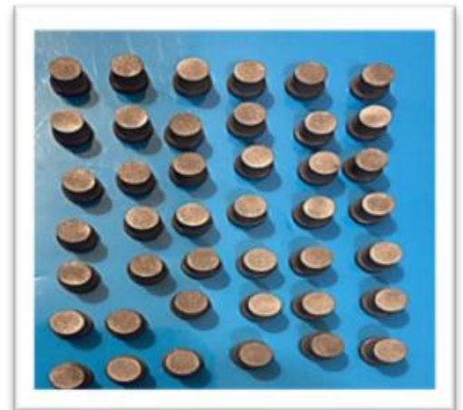
Fig. (5): The metal substructures' ultimate form uses five burs using a 5-axis milling unit.
