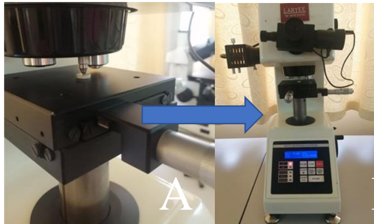
Fig. (8): A: Digital micro-Vickers hardness tester, B: Close-up view of a specimen on the stage of device
