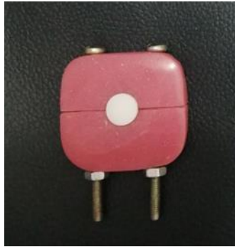
Fig. (7): Acrylic holder of specimens
