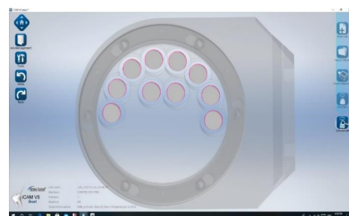
Fig. (3): Arranging the discs models on the blank
