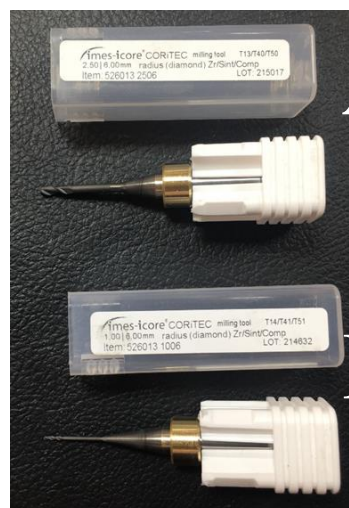
Fig. (6): Diamond burs used for milling procedure. A: 2.50 mm in diameter B: 1.00 mm in diameter
