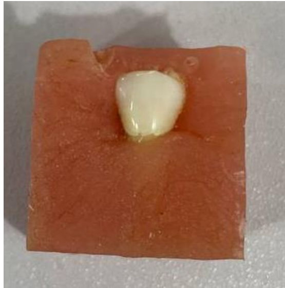
Fig. (1): Extracted Premolar mounted in acrylic.
