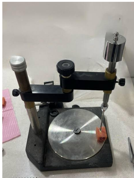
Fig. (2): Surveyor with 300 gm weight applied on the bracket.
