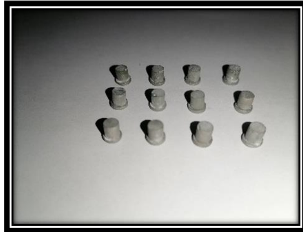
Figure (1): Nickle Chromium Metal samples.
