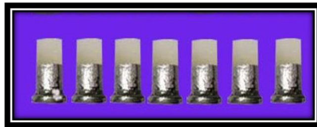
Figure (2) : Nickle Chromium Metal samples following ceramic build up.
