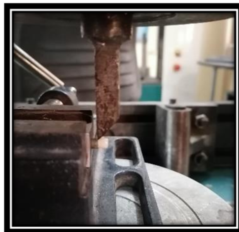
Figure (3): The sample in holder and mounted in a universal testing machine for shear bond strength test.
