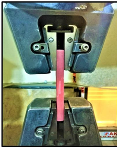
Fig. (6): Instron testing machine during test the shear bond strength specimen
