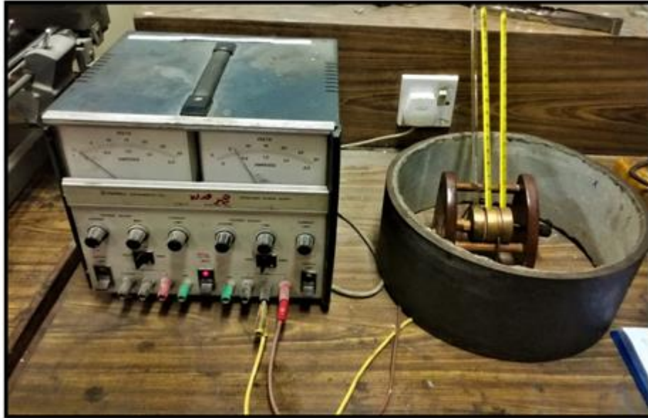
Fig. (2): Thermal conductivity apparatus (Lee disc)
