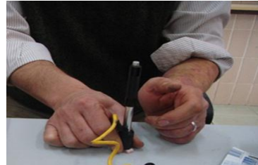
Fig. (4): Durometer hardness tester.
