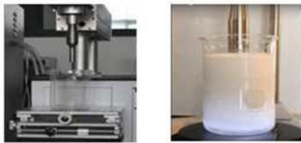
Fig. (3): Probe sonication apparatus.
