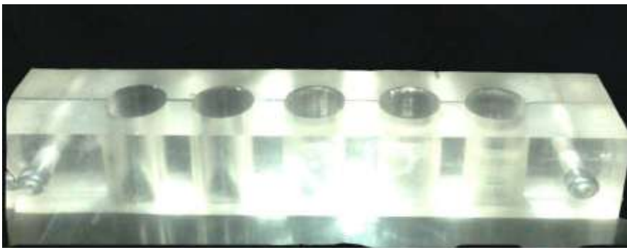
Figure (2): special split glass model used for preparation of compressive strength specimens.
