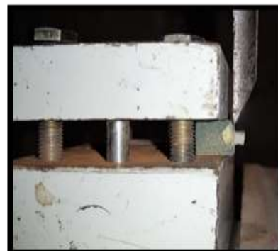
Fig. (8): Sample in special holding device and ready for shear test.
