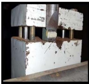
Fig.(7): Sample in special holding device and ready for shear test.
