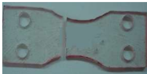
Fig.5. Fracture at the stressed region of unreinforced specimen
