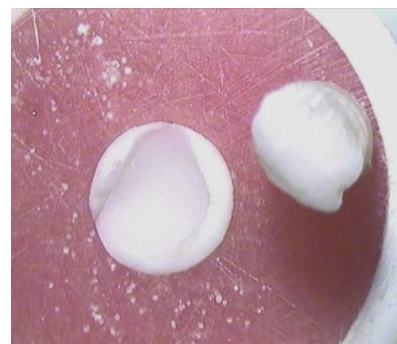
Fig.(4):- Cohesive failure within RMGIC.
