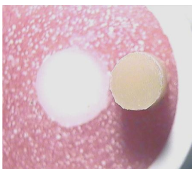
Fig.(3):- Adhesive failure.
