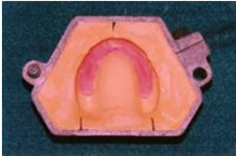
Fig.(17):- Molten wax poured into teeth mold
