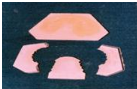
Fig.(14):- Stone parts of the upper half of flasking before forming the mold.
