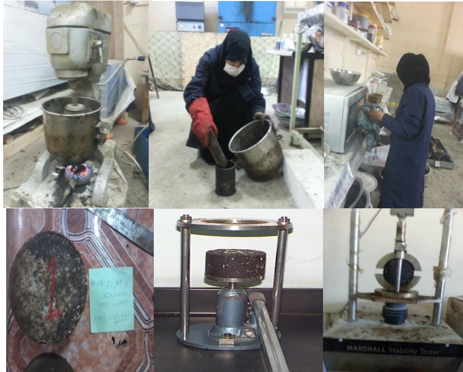
Figure 3. Preparation process for asphalt mixture.
