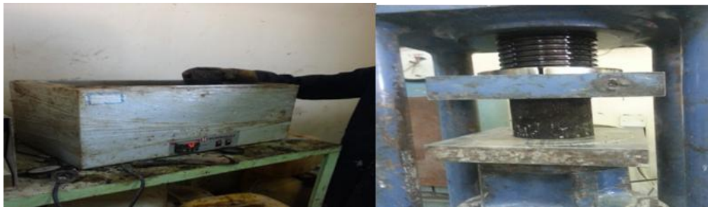
Figure 4. Compressive strength test.
