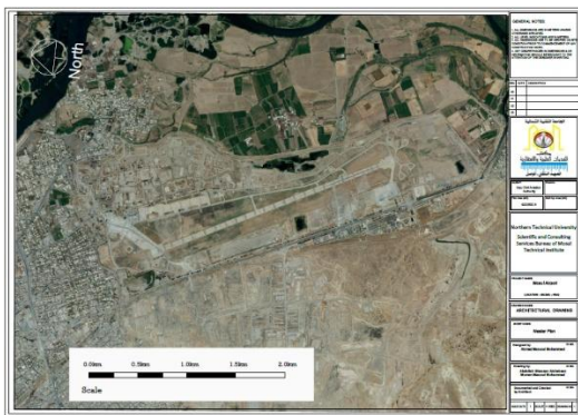
Map 1: Aerial photo of the new Mosul Airport. (Showing the scope of expansion for the length of the runway from the geographical south (right on the map) to exceed 3,000 meters). Source: https://www.pinterest.com/pin/827395762788865559/
