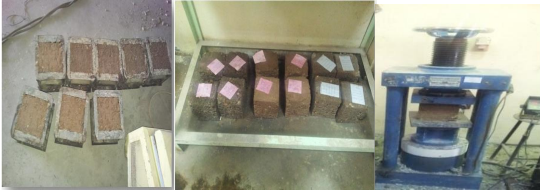
Figure 3: Preparation and Testing Procedures for unconfined compressive strength.
