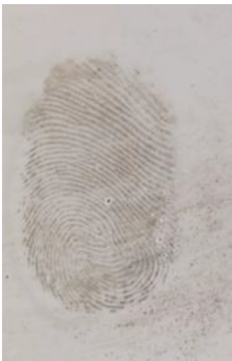
Fig. 7. Showing the latent fingerprint by the [Pd(DCPAC)_2]Cl complex on the aluminum surface.
