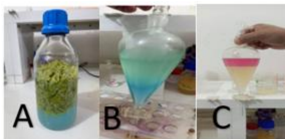
Figure (2) PNC extraction stage- (A)-Cutting cetrimide agar and putting in chloroform, (B)-Alkaline medium (NAOH), (C)- Acidic medium (HCL)
