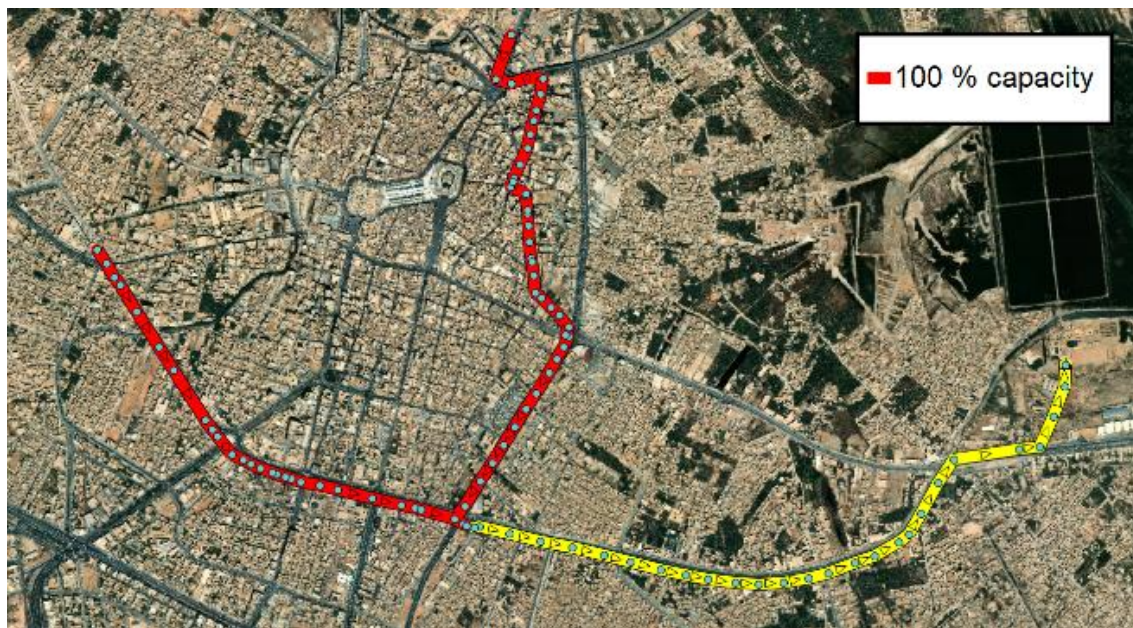
Figure 20. Pipe capacity situation under 25 mm/h rainfall event.
