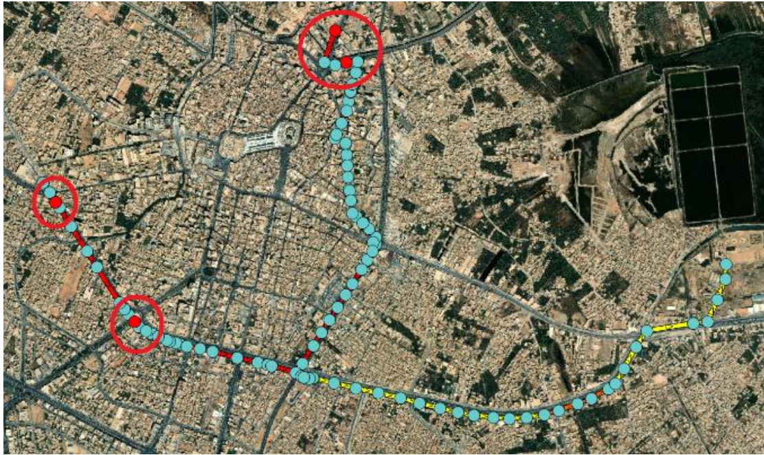
Figure 22. Flooding places (30 mm/h rainfall event).
