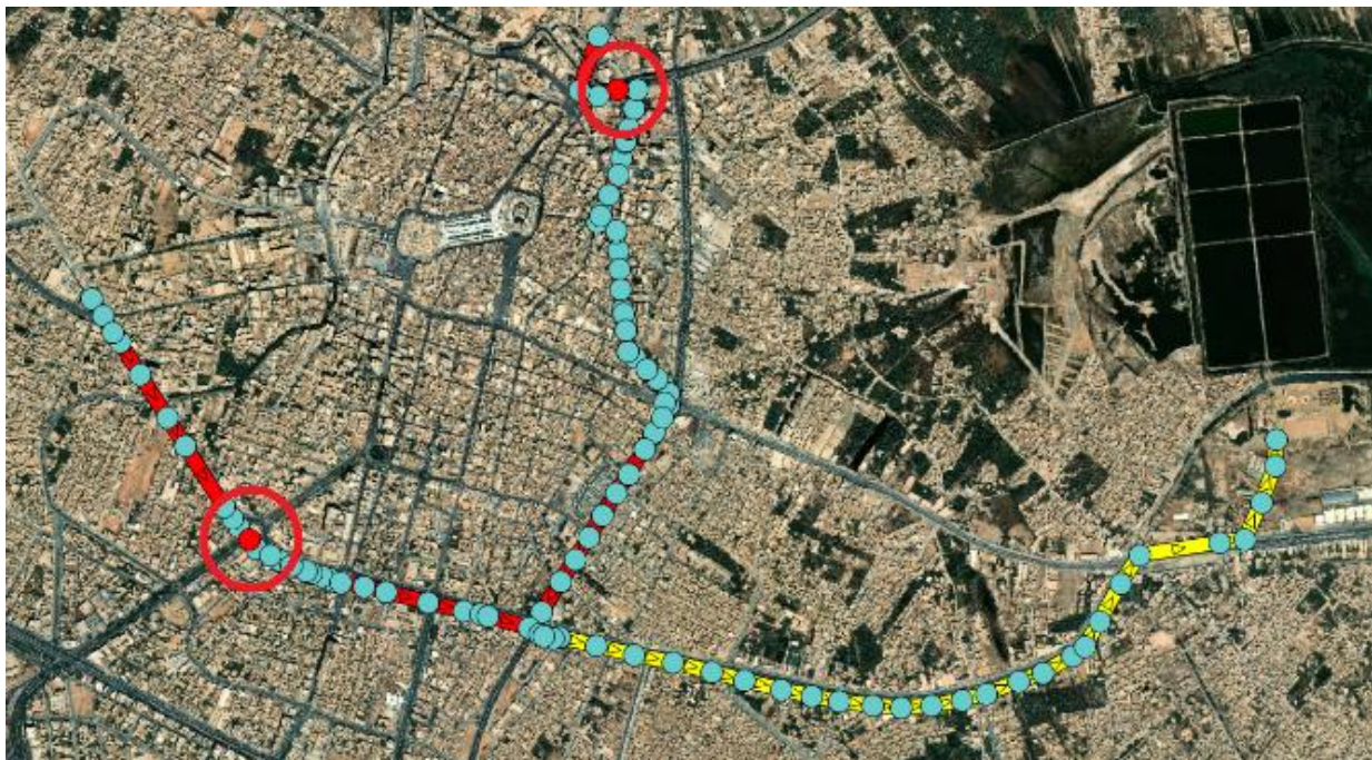
Figure 19. Flooding places (25 mm/h rainfall event).
