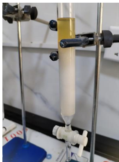
Figure 4: Extraction of Biosurfactant by silica column chromatography technique
