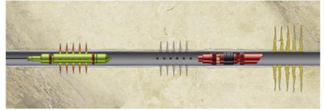
Figure (2) the mechanism of operation of the oil shale perforation technique using a wire tractor
