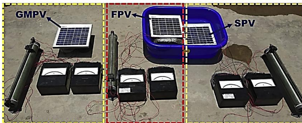
Figure 2. An experimental configuration of a solar module using submerged, floating, and ground-mount installation techniques [22]
