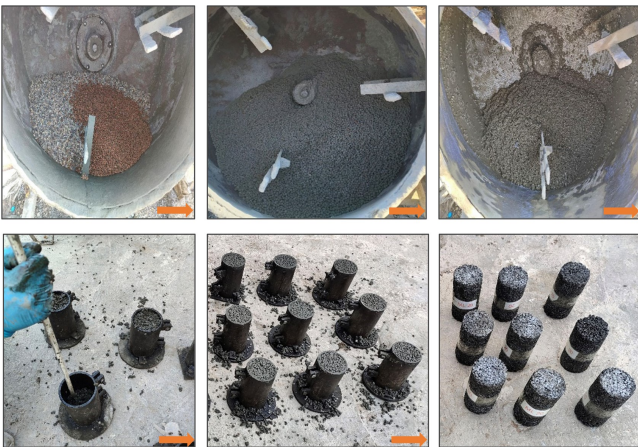
Figure 3. Pervious concrete mixing and casting process.
