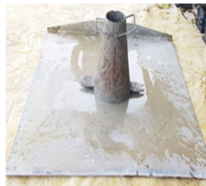
(b) Slump flow
