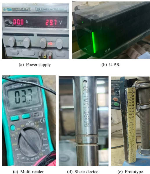
Figure 10. (a) D.C. power supply, (b) U.P.S. power supply, (c) Digital multi-reader electrical measurement, (d) Vane shear device, (e) Pile concrete shaft (graduated) prototype.
