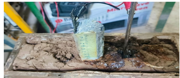
Figure 12. Following the completion of the pile driving process with electro-osmosis (E.O.) enhancement, the pile shaft prototype is depicted with the red wire indicating the anode and the black wire representing the cathode.
