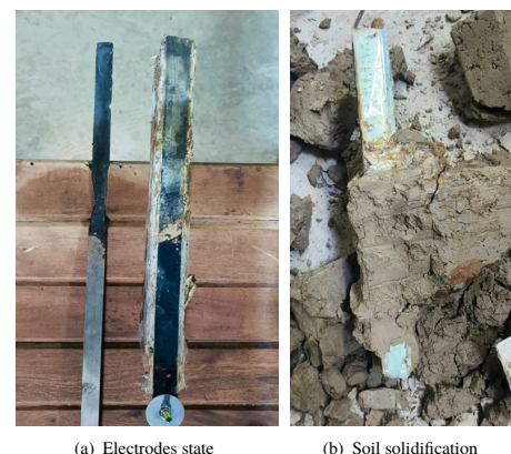
Figure 13. (a) Electrodes state due to E.O. subjecting for about (48) hours, (b) Soil solidification mass around the pile prototype shaft due to E.O. subjecting for about (48) hours.
