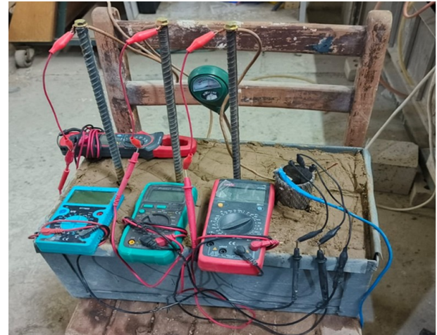
Figure 11. Horizontal E.O. soil container, E.O. electrodes, and voltmeters.
